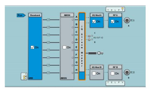
The R&S\*SMW200A is the ideal generator for multistandard radio and interference tests. In this example, it is generating eight different frequency-spaced signals that are added up in real time for receiver testing.
