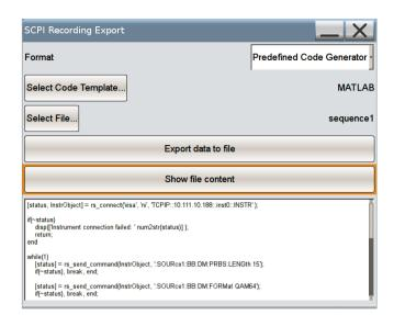
The built-in SCPI macro recorder and code generator supports fast, convenient generation of SCPI program sequences.
