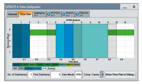
Time plan display in the LTE option of the R&S®SMW200A.
