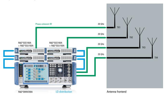
Setup with a two-path R&S\*SMW200A, two R&S\*SGS100A and two R&S\*SGU100A to generate four phase-coherent CW or modulated signals, for example for antenna testing up to 20 GHz. The setup can be scaled to 40 GHz and duplicated if more RF paths are required.
