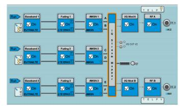
Block diagram of the R&S®SMW200A configured for the generation of a LTE Release 11 felCIC test scenario. One R&S®SMW200A simultaneously generates the LTE serving cell as well as the two aggressor cells, each with 2x2 MIMO, with correlated fading channels.
