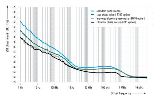
Measured SSB phase noise performance at f=1 GHz, CW mode, standard performance versus the R&S $^{\circ}$ SMW-B709, R&S $^{\circ}$ SMW-B710 and R&S $^{\circ}$ SMW-B711 options.
