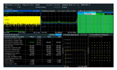
Measured EVM of a 5G NR signal (100 MHz channel bandwidth, 640AM PDSCH, 39 GHz carrier frequency).
